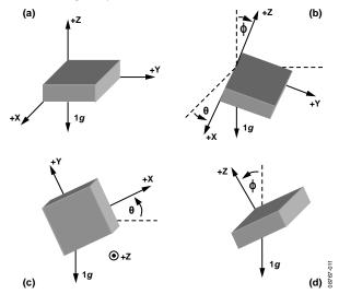
Figure 11. Angles of Spherical Coordinate System
