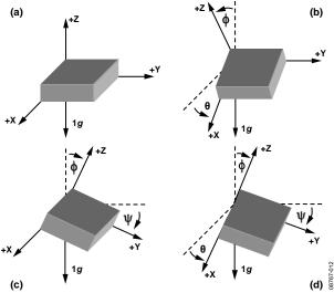
Figure 12. Angles for Independent Inclination Sensing
