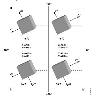
Figure 10. Angle of Inclination and Sign of Acceleration for Ouadrant Detection
