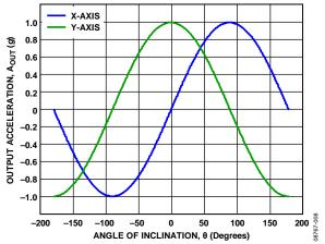
Figure 8. Output Acceleration vs. Angle of Inclination for Dual-Axis Inclination Sensing
