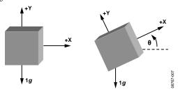
Figure 7. Two Axes Used for Tilt Sensing
